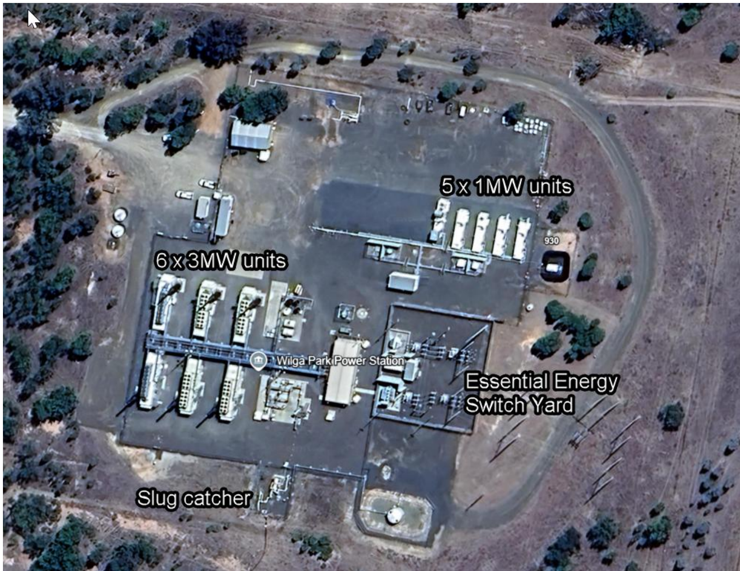
Figure 1.1 Wilga Park Power Station site layout
