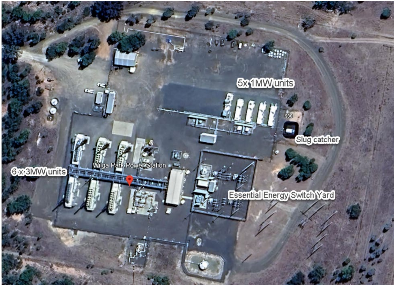
Figure 2.1 Wilga Park Power Station site layout
