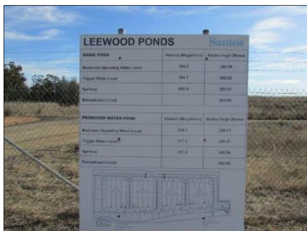
Photo 3 – Leewood ponds volume (ML) and relative height (m) (22 August 2023)
