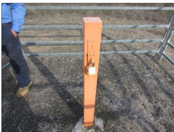
Photo 33 – Example of seepage detection bore (LWDSDB03) at the Leewood Produced Water ponds (22 August 2023)
