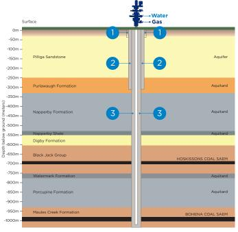
1 Steel conductor inserted and cemented into place
