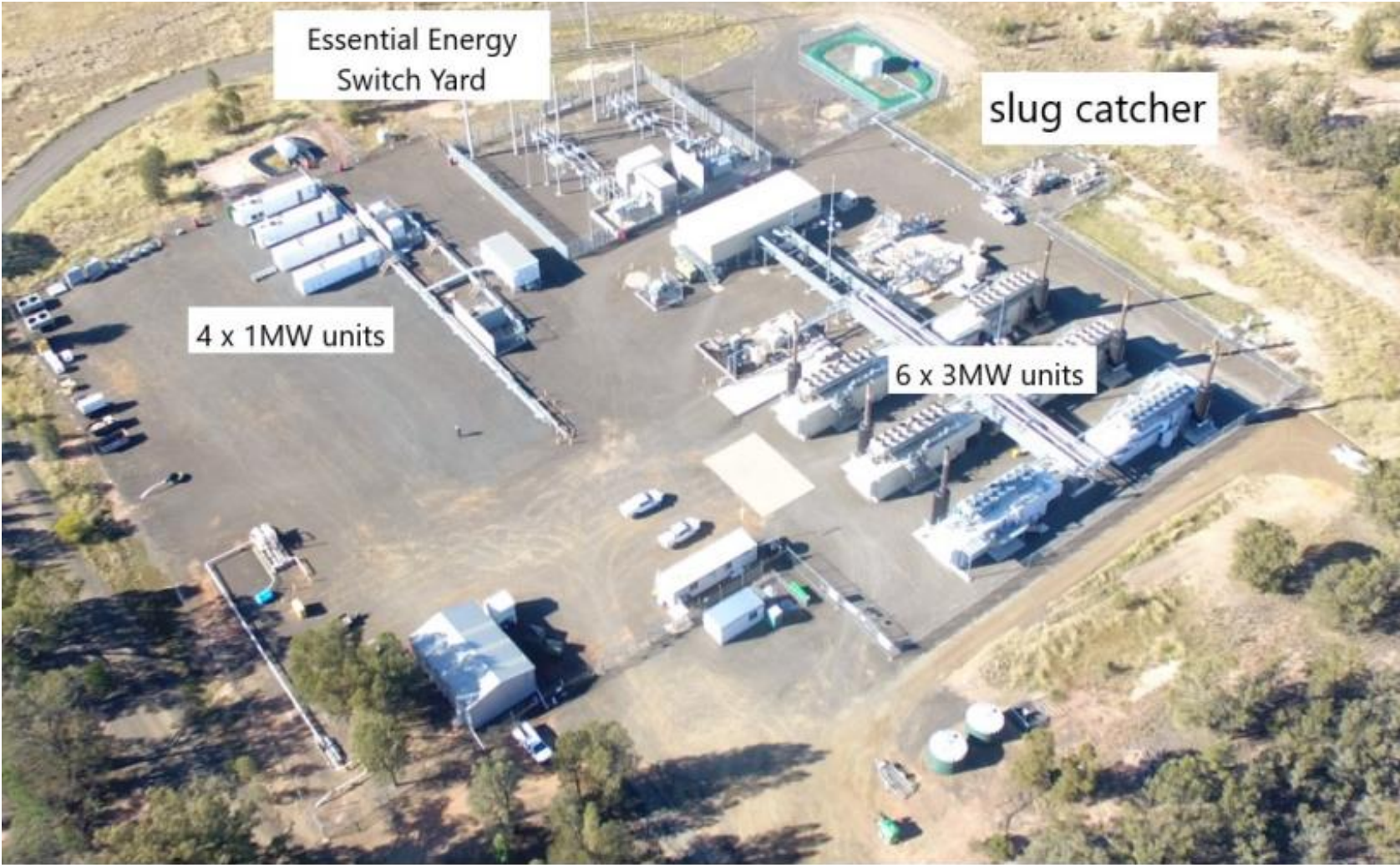
Figure 2.1 Wilga Park Power Station layout
