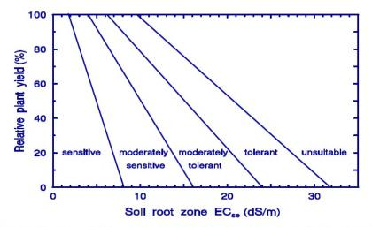
Figure 9.2.4 Relative crop yield in relation to soil salinity (EC<sub>se</sub>) for plant salt tolerance groupings of Maas and Hoffman (1977). Note that 1 dS/m = 1000 μS/cm.
