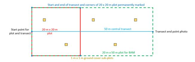
Figure 12.1 - Example of rehabilitation monitoring plot configuration
