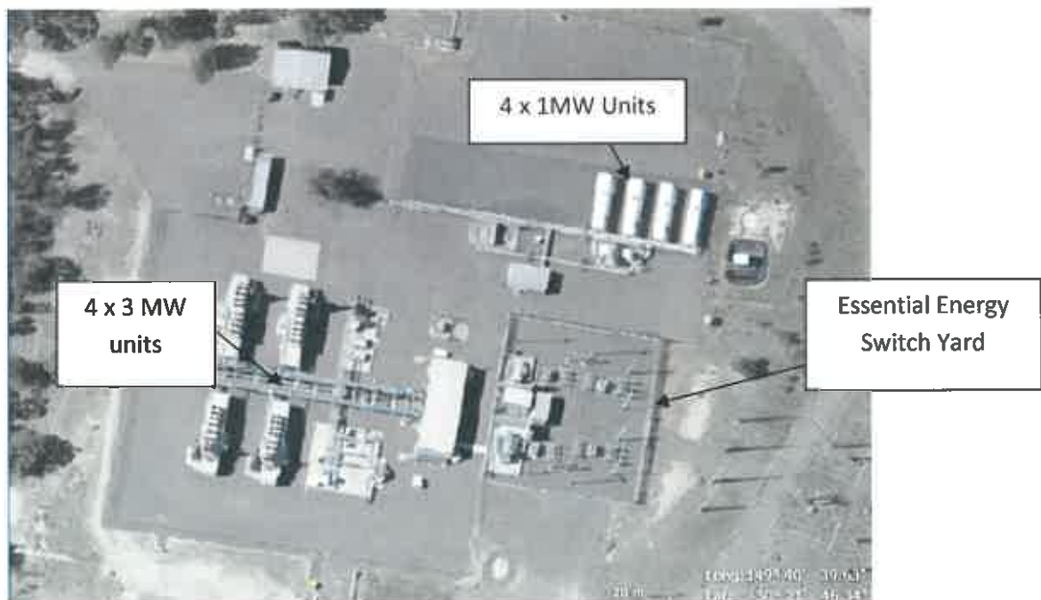
Figure 1: Wilga Park Power Station Layout
