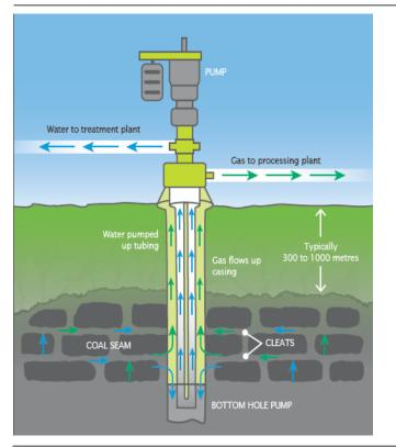
Figure 2.1 CSG production process
