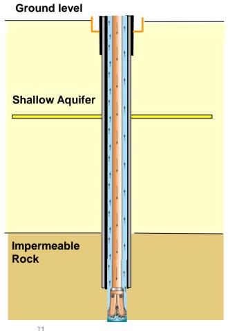
216 mm diameter hole is drilled through a series of impermeable rock layers before finishing above the targeted coal.
