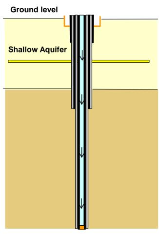
178 mm diameter steel casing is run into the hole
