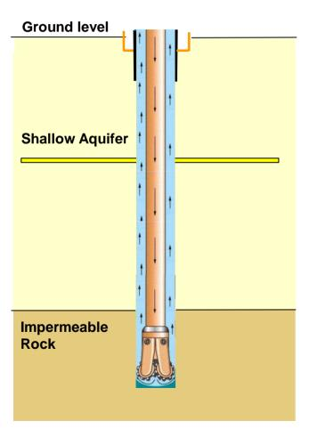
355 mm steel conductor is cemented into competent rock, 10 m below ground level
