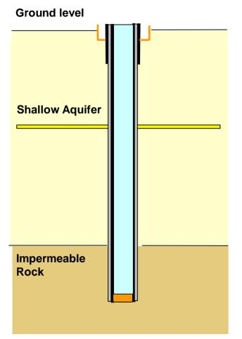
244 mm steel casing is run into the hole
