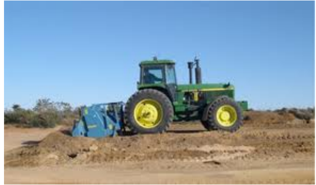
Plate 4. Tractor aerating contaminated soil
