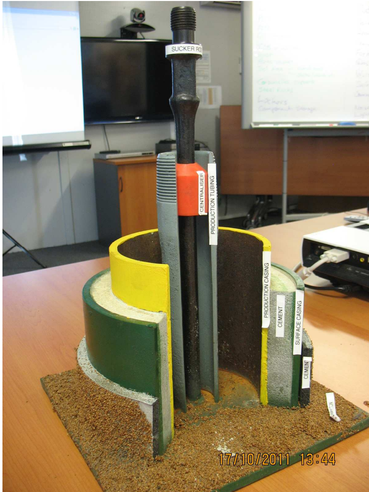
Section of casing AGL Camden Gas
