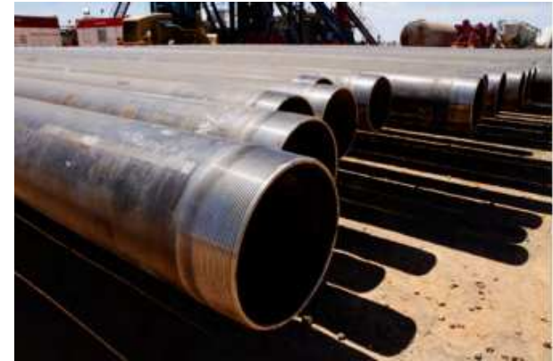
Example of steel casing
