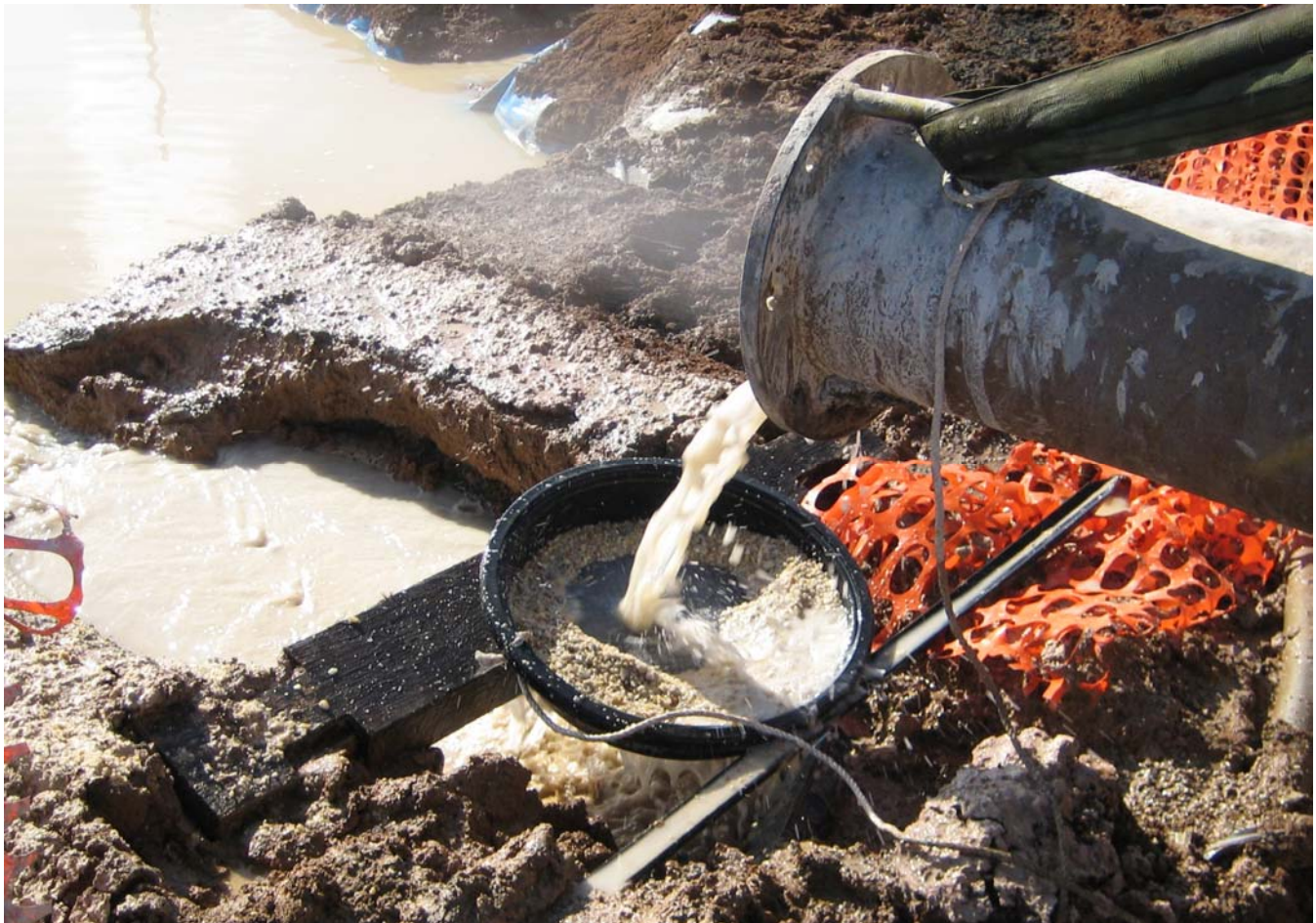
Figure 14 Drilling fluid and drill cuttings exiting the mud system (PEL433 Allambi-1C)
