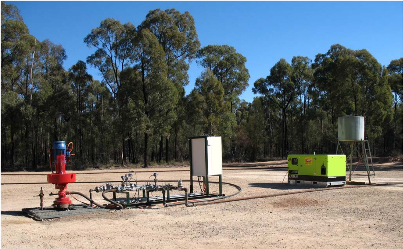
Figure 12 Typical surface installation required to operate a CSG well
