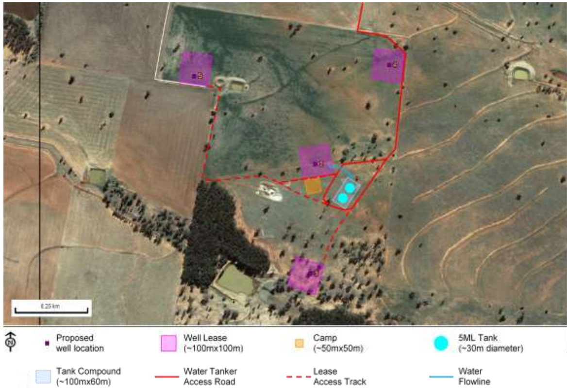
Figure 4.3: Aerial Photograph Kahlua 2 Well site and Water Storage Facilities
