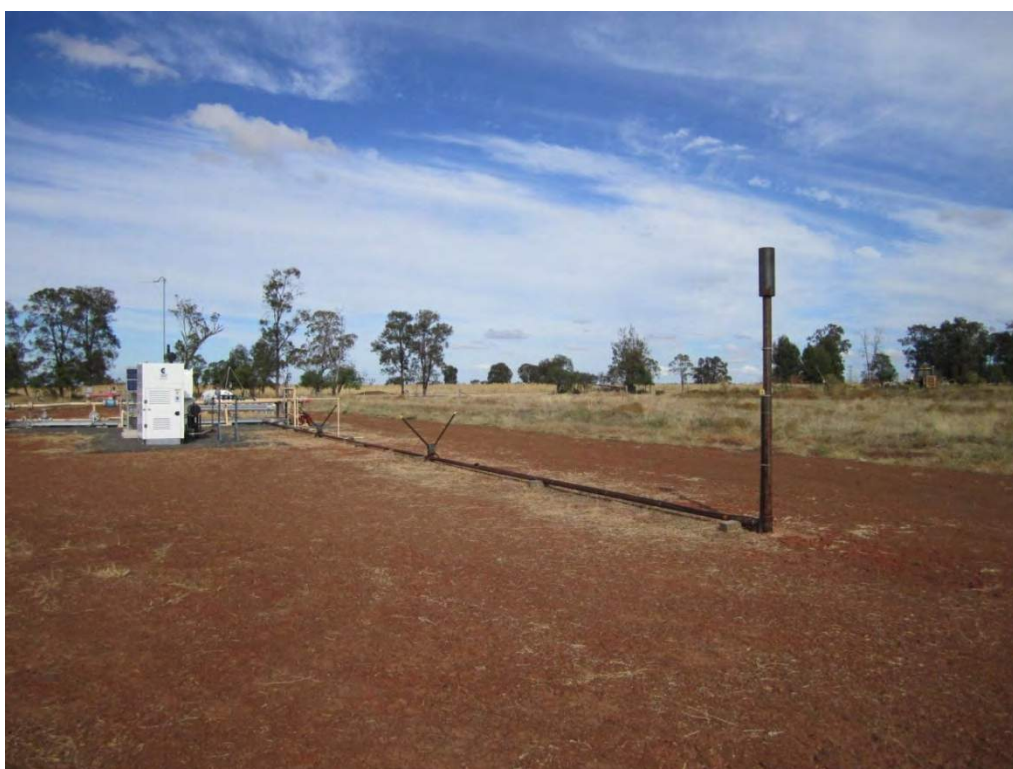
Plate 2-2 Typical flare assembly
