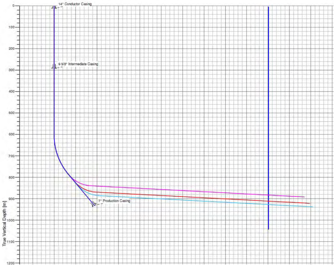
Figure 2-5 Well schematic – indicative example of directional and vertical pilot well interception
