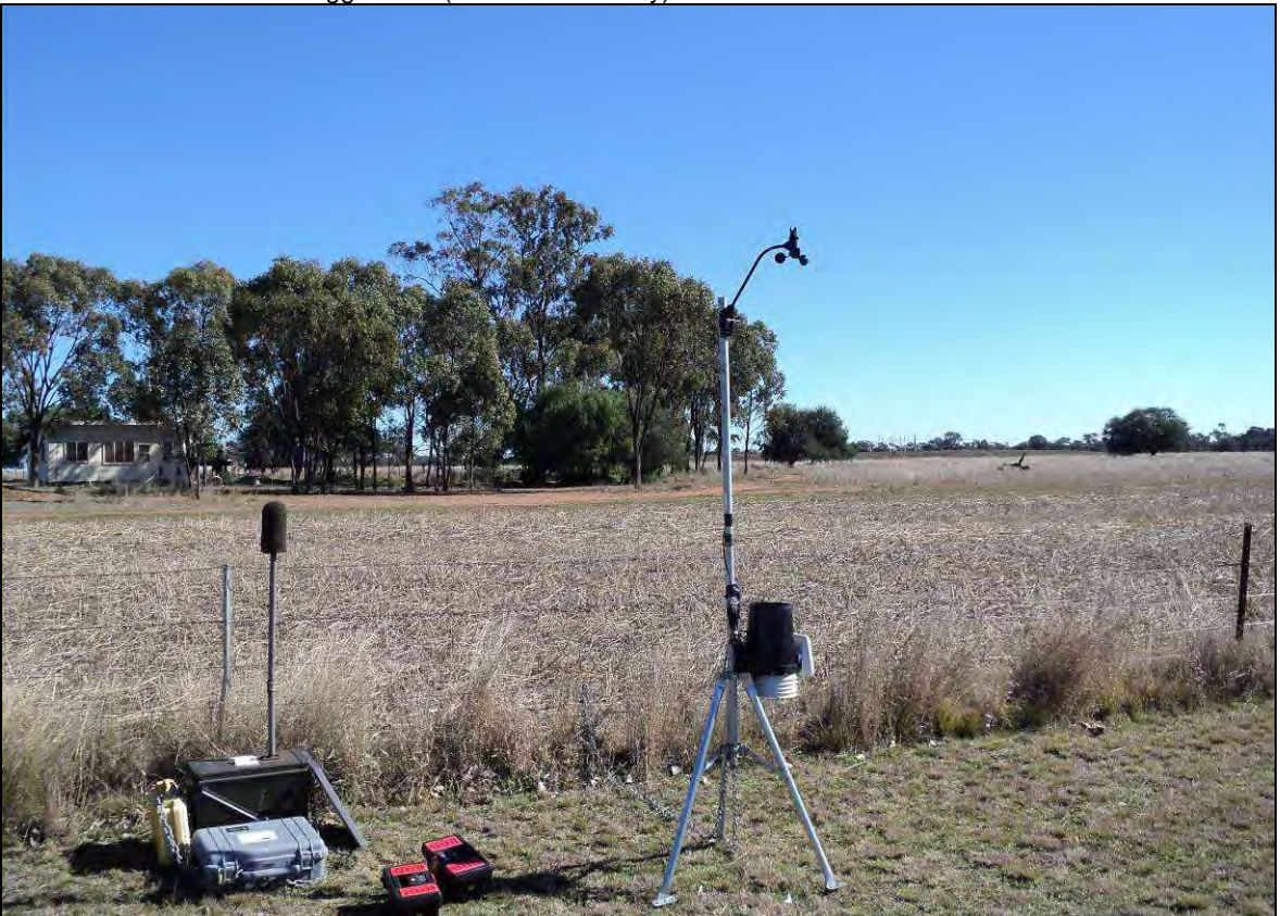
Photo 2.4: View of noise logger ML4 (June 2012 Survey).
