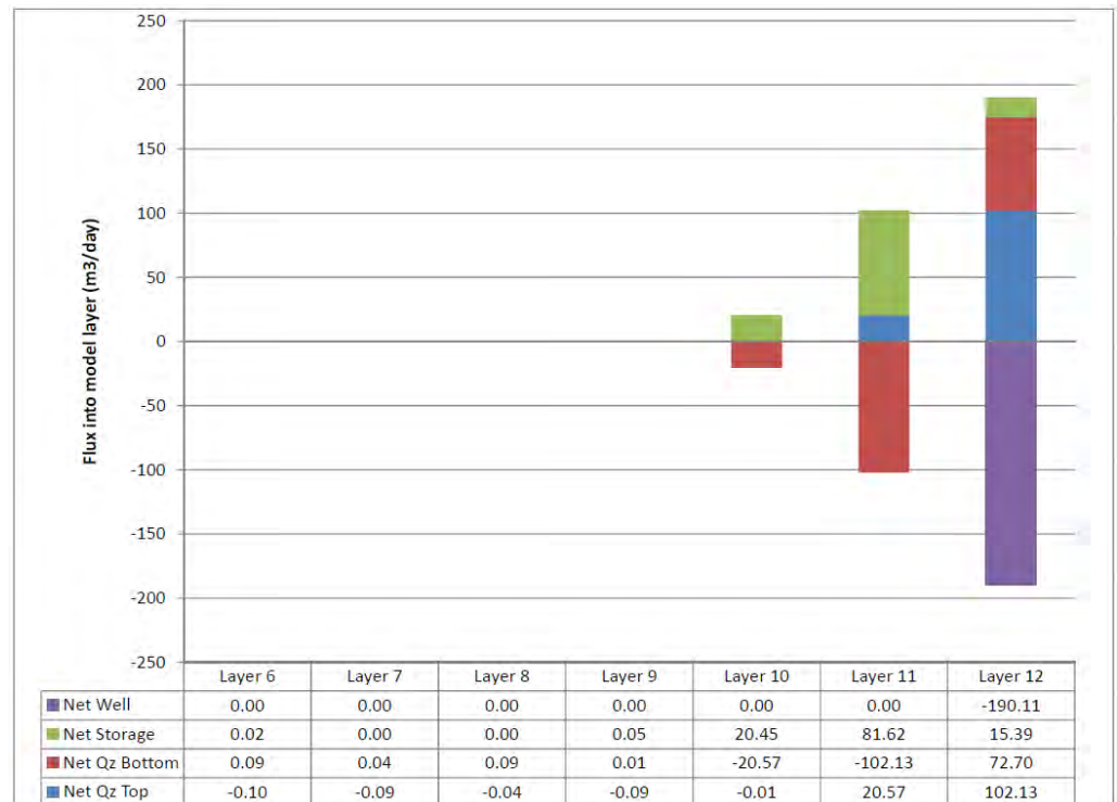
Figure 5-3: Mass balance summary by model layer, 3 years from start of pilot (Simulation DWH26_29_wel)
